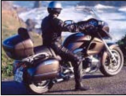
The upper edge of the screen is not in the line of vision. This is a particular advantage when riding in rain or if the windscreen becomes dirty on long journeys. (An even shorter screen is available as an optional extra.) In addition, the rider can control the degree of wind deflection and protection by opening additional air deflectors if the weather worsens.
