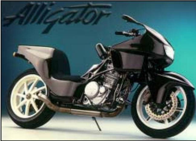
placed below the handlebars. The gas tank is mounted below the seat and behind the engine.
